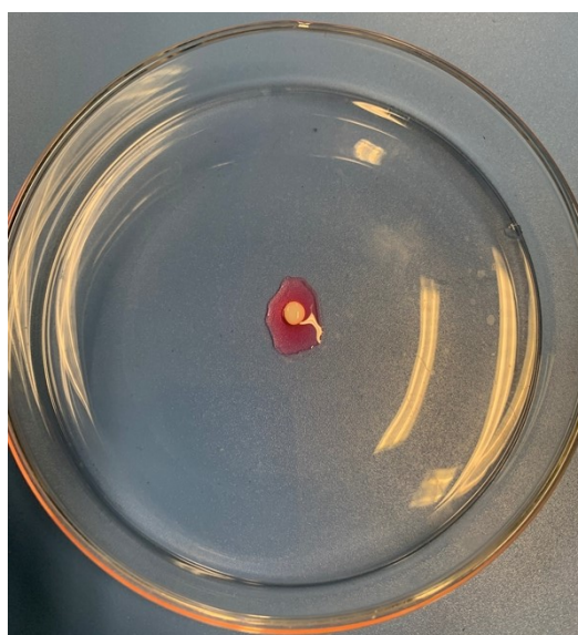
Fig. S9 Digital photo of emulsion stabilized by CQDs- C_{18}N in the presence of lipophilic Nile red in toluene, indicative of the formation of oil-in-water emulsion.
