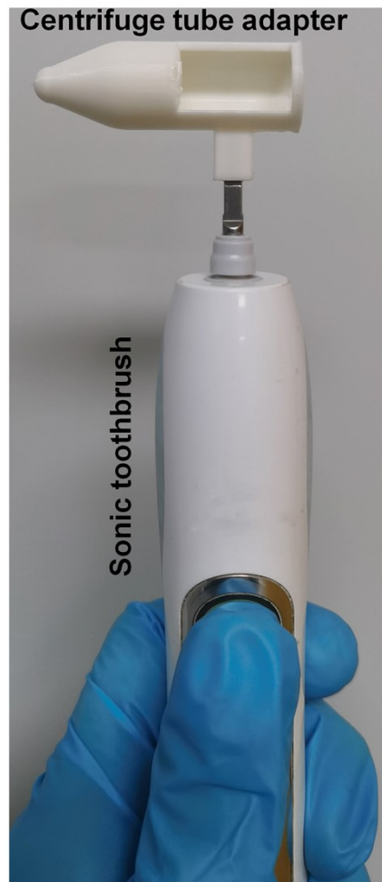
Fig.S1 Sonic vibration extraction device
