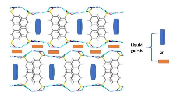
Guanidinium—biphenyldisulfonic acid (GBPS) were used as a coformer for the cocrystallization of liquid compounds **1-8** and get their structures determined by single crystal X-ray diffraction.
