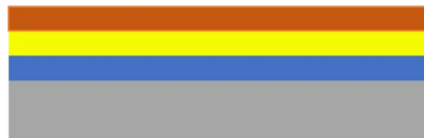
Figure S2: (a) – (c) Schematic of Ag/Cu, Au/Cu, and Ag/Au/Cu metal films by sputtering. Subscripts indicate the multilayer thickness.
