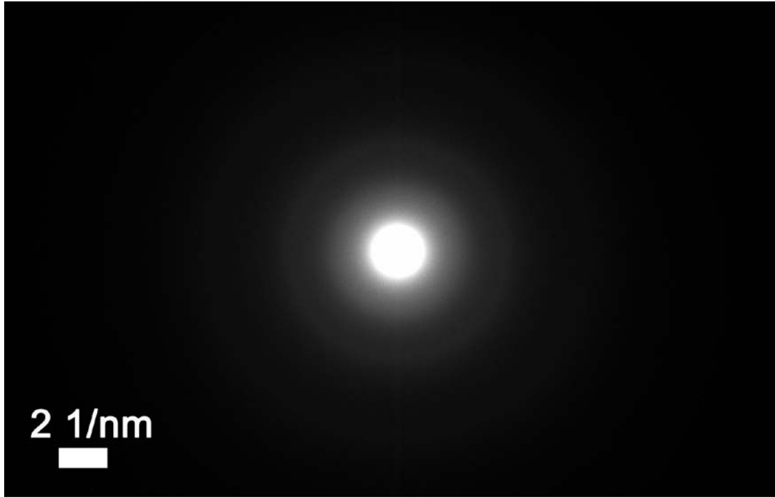
Figure S3. electron diffraction pattern image of the cal-FeZIF-NSC-0.2 composite.
