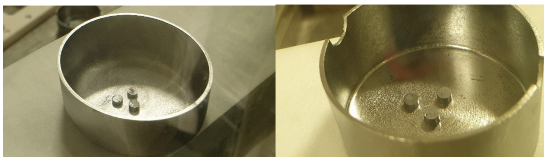
Fig. S2 Pictures of the sintered disks: U 0.90 Am 0.10 O 2 (left) and U 0.80 Am 0.20 O 2 (right)
