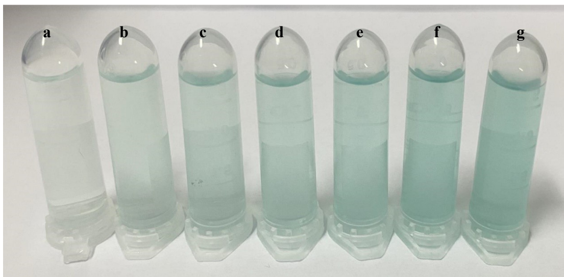
Figure. S4. The gradually deepened color of dispersion containing TMB and \text{H}_2\text{O}_2 along with the increased concentration of Sc-MOF nanozyme from 0 to 50 \text{ mg L}^{-1} , a-g: 0, 0.5 \text{ mg L}^{-1} , 2 \text{ mg L}^{-1} , 5 \text{ mg L}^{-1} , 10 \text{ mg L}^{-1} , 25 \text{ mg L}^{-1} and 50 \text{ mg L}^{-1} .
