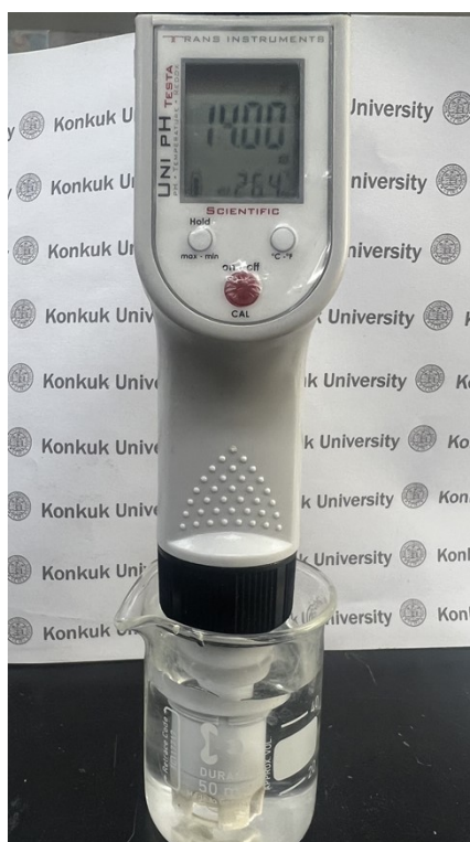
Figure S6. Photograph image measuring pH of 1M KOH electrolyte.
