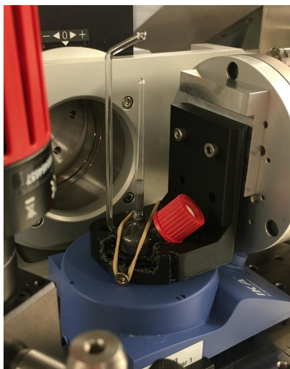
Fig. S8. Hydrogenated \text{Bi}_{24}\text{O}_{31}\text{Br}_{10} in isopropanol suspension in the LRC in argon atmosphere after illumination on Balder at the MAX IV Laboratory. The sample prior to irradiation is shown in Fig. 2d in the manuscript.
