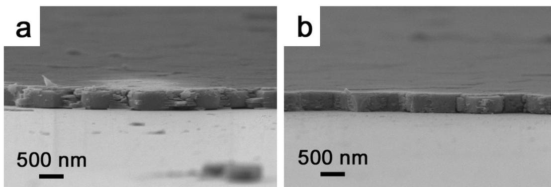
Figure S2 Cross-sectional SEM images of MFI zeolite films synthesized in mixtures with composition: (a) 0.2TPAOH : 1TEOS : 200H<sub>2</sub>O : 0.6-(1,3-)C<sub>6</sub>H<sub>6</sub>O<sub>2</sub> and (b) 0.2TPAOH : 1TEOS : 200H<sub>2</sub>O : 1.0-(1,4-)C<sub>6</sub>H<sub>6</sub>O<sub>2</sub>.
