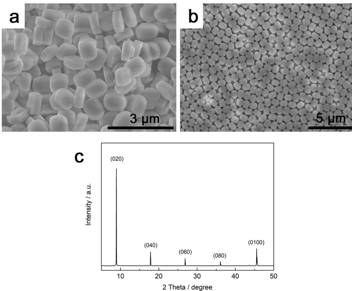
Figure S1 SEM image of (a) zeolite MFI seeds and (b) their monolayer on stainless steel support.
