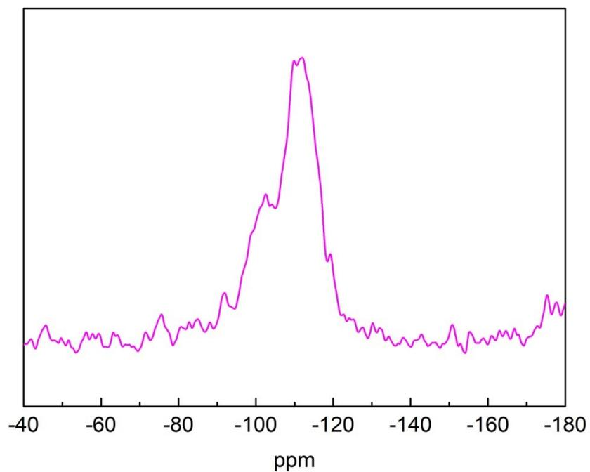
Figure S8 Solid-state  $^{29}\text{Si}$ -NMR of the precipitate synthesized at  $165^\circ\text{C}$  for 2 h. Synthesis mixture composition: 0.2TPAOH: 1TEOS : 200 $\text{H}_2\text{O}$ : 0.6(1,3-)C $_6$ H $_6$ O $_2$ . Scanning time: 10.5 hours.
