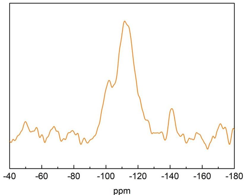
Figure S7 Solid-state  $^{29}\text{Si}$ -NMR of the precipitate synthesized at  $165^\circ\text{C}$  for 2 h. Synthesis mixture composition: 0.2TPAOH: 1TEOS : 200 $\text{H}_2\text{O}$ : 0.3(1,2-)C $_6\text{H}_6\text{O}_2$ . Scanning time: 2 hours.
