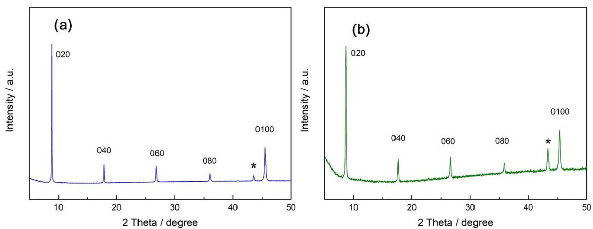
Figure S4 XRD patterns of calcined films in Fig. 1c (a) and 1g (b). (\*) Peaks from the SS plate.
