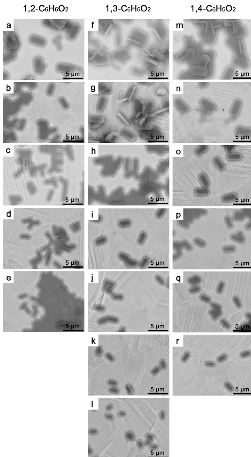
Figure S5 MFI zeolite crystals at the edge of the films synthesized with different molar amounts of dihydroxy-benzene isomers, left column: 1,2-C<sub>6</sub>H<sub>6</sub>O<sub>2</sub> (a-0.1, b-0.2, c-0.3, d-0.4, e-0.5), middle column: 1,3-C<sub>6</sub>H<sub>6</sub>O<sub>2</sub> (f-0.1, g-0.3, h-0.4, i-0.5, j-0.6, k-0.8, l-1.0), right column: 1,4-C<sub>6</sub>H<sub>6</sub>O<sub>2</sub> (m-0.1, n-0.3, o-0.5, p-1.0, q-1.2, r-1.5).
