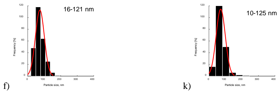
Fig. S1 Particle size distribution determined from SEM: a) Bindzil ( B100-P ), b) H-MCM-41 ( M100-P ), c) H-MCM-41 with 10% Bindzil ( B10M90-P ), d) H-MCM-41 with 25% Bindzil ( B25M75-P ), e) H-MCM-41 with 30% Bindzil ( B30M70-P ), f) H-MCM-41 with 50% Bindzil ( B50M50-P ), g) H-MCM-41 ( M100-E ), h) H-MCM-41 with 10% Bindzil ( B10M90-E ), i) H-MCM-41 with 25% Bindzil ( B25M75-E ), j) H-MCM-41 with 30% Bindzil ( B30M70-E ), k) H-MCM-41 with 50% Bindzil ( B50M50-E ).
