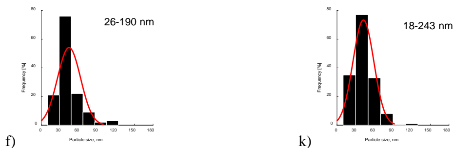
Fig. S2 Particle size distribution determined from TEM: a) Bindzil ( B100-P ), b) H-MCM-41 ( M100-P ), c) H-MCM-41 with 10% Bindzil ( B10M90-P ), d) H-MCM-41 with 25% Bindzil ( B25M75-P ), e) H-MCM-41 with 30% Bindzil ( B30M70-P ), f) H-MCM-41 with 50% Bindzil ( B50M50-P ), g) H-MCM-41 ( M100-E ), h) H-MCM-41 with 10% Bindzil ( B10M90-E ), i) H-MCM-41 with 25% Bindzil ( B25M75-E ), j) H-MCM-41 with 30% Bindzil ( B30M70-E ), k) H-MCM-41 with 50% Bindzil ( B50M50-E ).
