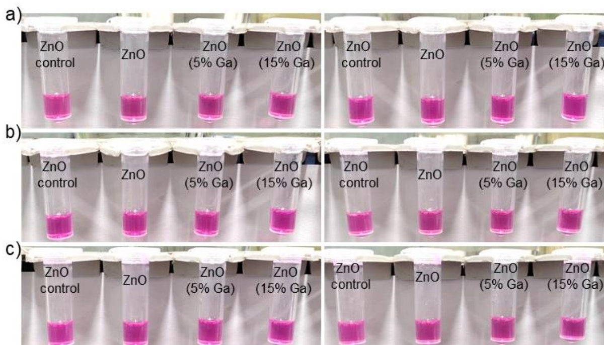
Figure S8. Colloidal stability of zinc oxide nanoparticles of different concentrations in cell culture media taken at different time interval. a) 0.1 mg/mL, b) 0.2 mg/mL and c) 0.4 mg/mL (left: 0 h, right: after 24 h) Results indicate the nanoparticles are stable in cell culture media without any precipitation.
