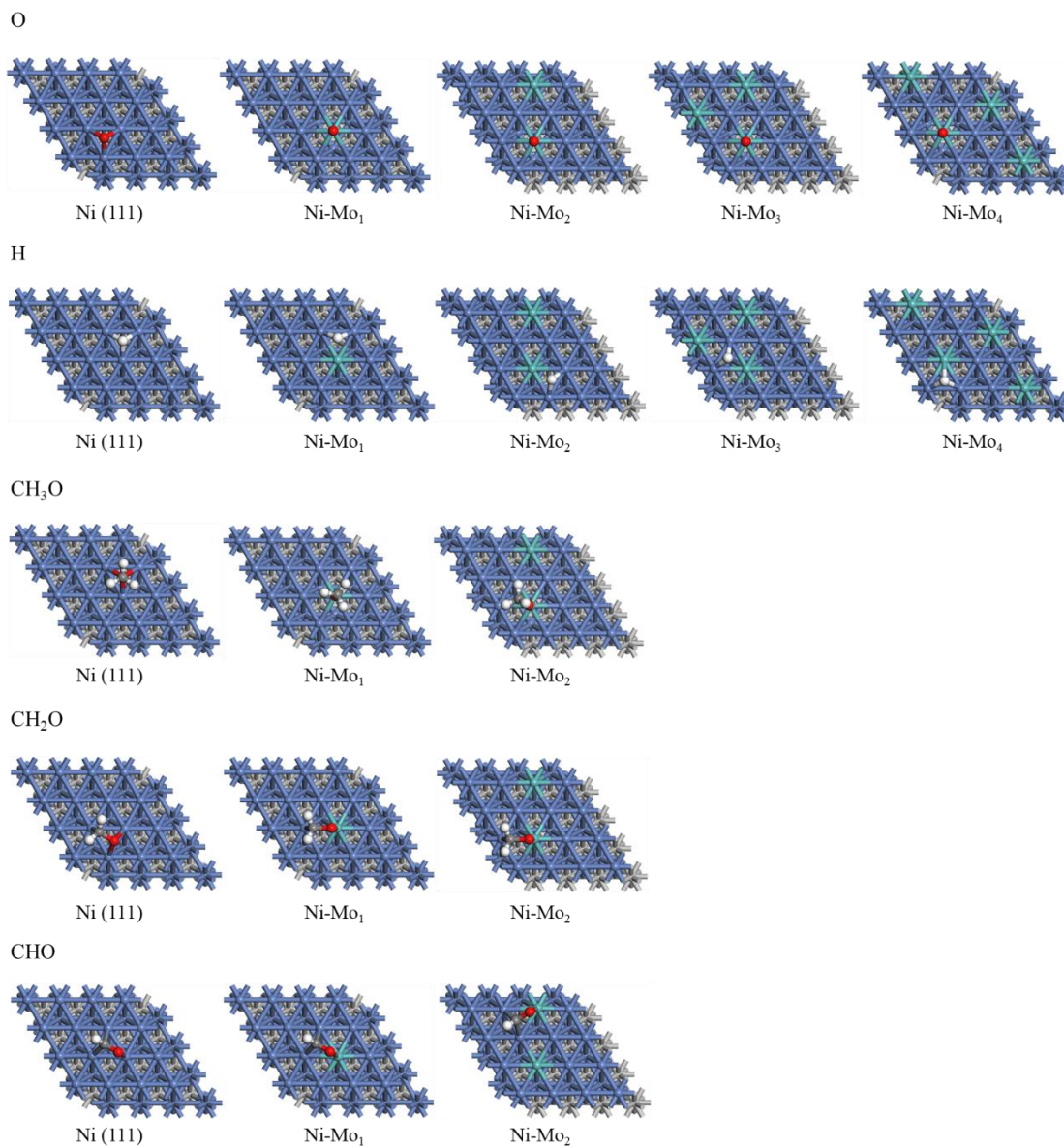
Fig. S3 The most stable configurations of the DRM species on the Ni/Mo. The red, white and dark gray balls denote the O, H and C atoms, respectively.
