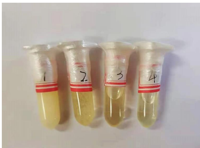
Fig. S5. The phase change of BmimCl-TAA (1:1) in absorption process of HCl gas
