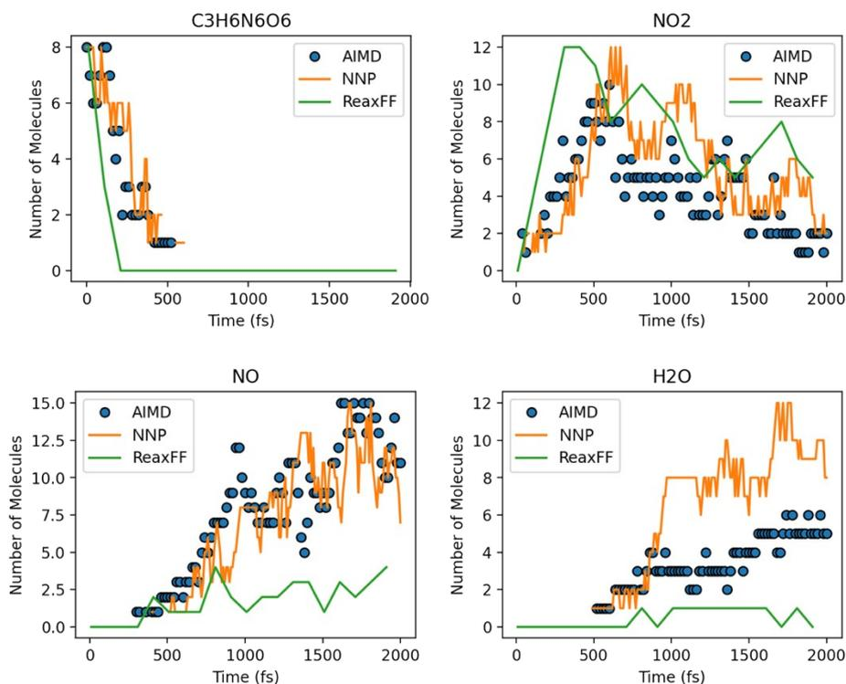
Fig. S3 Evolution of the major species (RDX,  $\text{NO}_2$ ,  $\text{NO}$  and  $\text{H}_2\text{O}$ ) during the initial decomposition process predicted by AIMD, NNP, and ReaxFF models.
