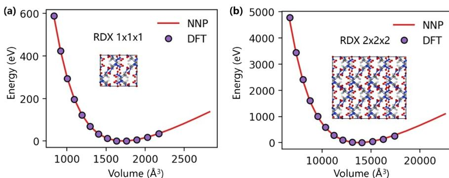
Fig. S2 Equation of state curve for (a) RDX unit cell and (b) 2x2x2 supercell predicted by NNP and DFT methods. The NNP is trained on the RDX unit cell datasets.
