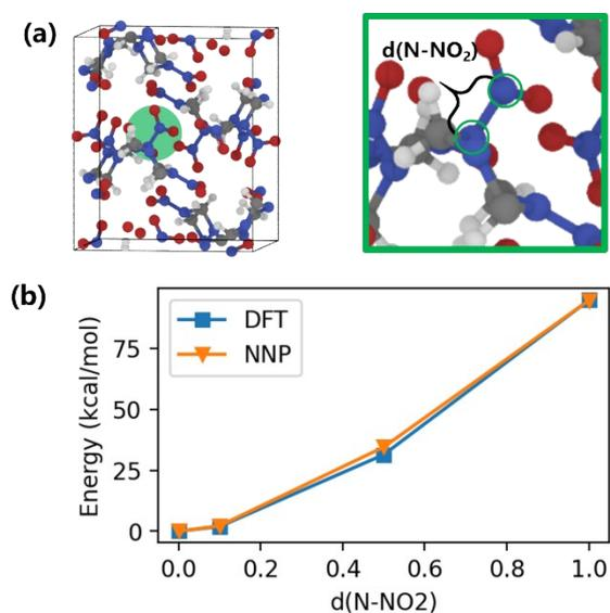
Fig. S1 (a) Illustration of N-N homolysis in bulk RDX crystal, (b) the potential energy surface of N-N homolysis in bulk RDX crystal predicted by DFT (PBE/DZVP-MOLOPT) and NNP.
