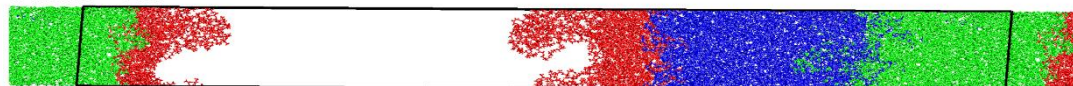
Fig. S7. Evolution of the systems during uniaxial deformation along the direction normal to the PLA/PBS interface (green, red, and blue colors are PLA, compatibilizer, and PBS chains, respectively). The black arrow indicates the region where the fracture initiates.
