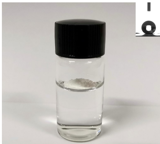
Fig. S1 Behavior of PDVB/SiO 2 in water and the contact angle analysis.
