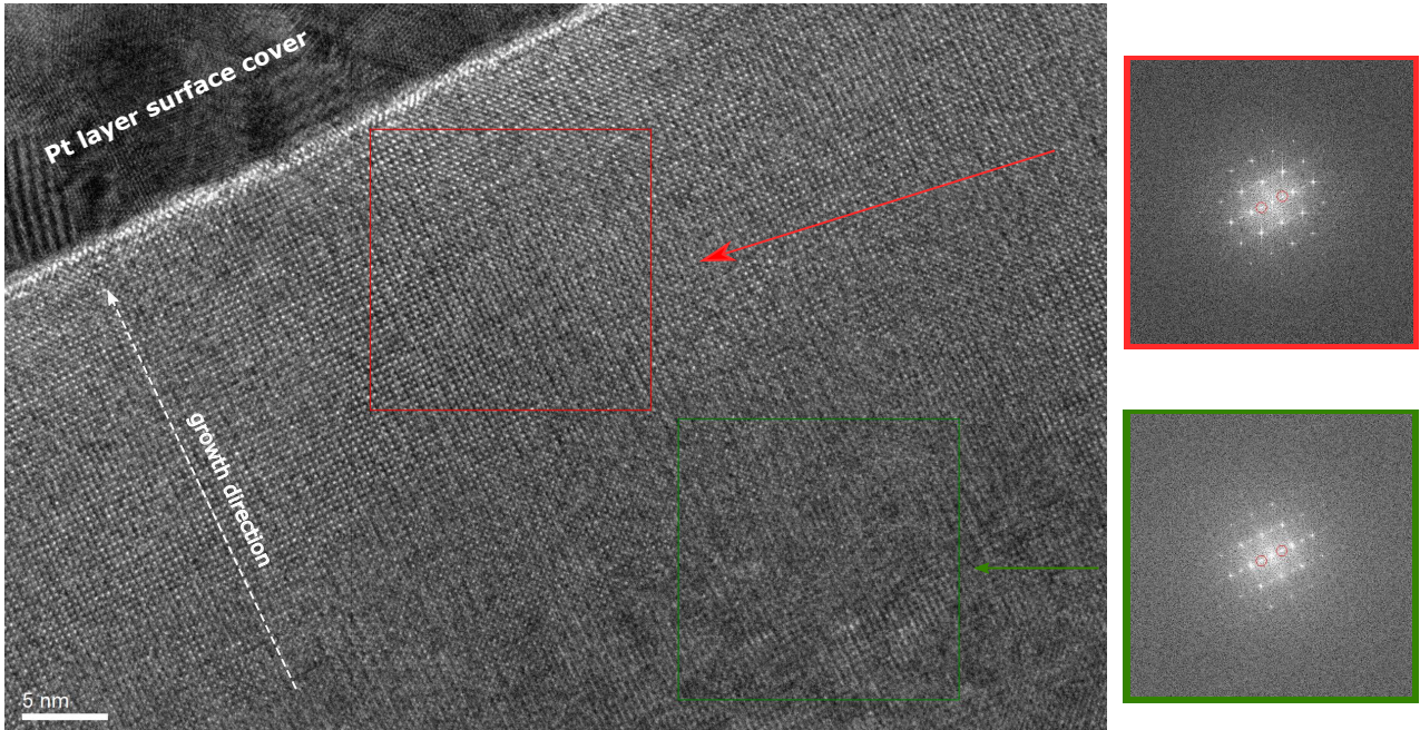
Figure 3: FFT analysis of LSF thin film. Red circles in the FFT patterns highlights the half-integer reflections indicating the presence of the brownmillerite phase.
