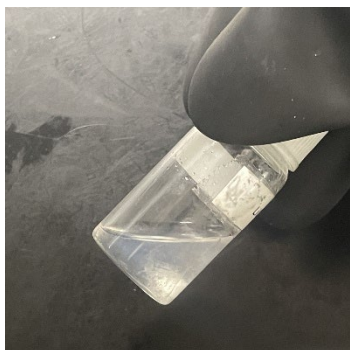
Figure S1. Photograph of a [\text{LiFSA}]/[\text{SL}]/[\text{HFE}] = 1/2.5/3 mixture after storage for several weeks at room temperature.
