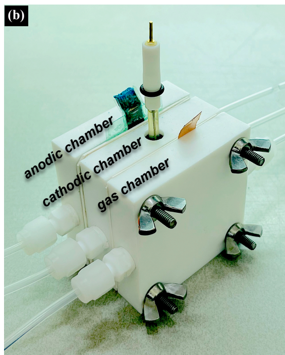
Figure S1. Comparison of the flow cell for (a) the operando X-ray absorption spectroscopy and (b) the typical electrochemical measurement.
