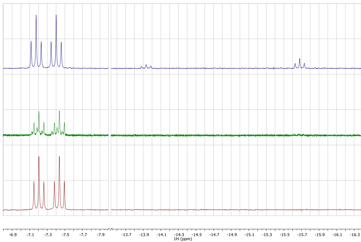
Figure S38. Stacked 1 H NMR spectra (hydride region) for the transformation of complex 2 under H 2 /CO 2 gas in THF-d 8 . Note the gradual transformation of 2
