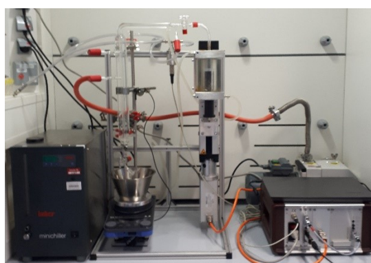
Figure S17. Scheme and picture of the peroxide decomposition set-up used for the simulation of hydroperoxide decomposition during cyclohexene oxidation using \text{H}_2\text{O}_2 and tert -butyl hydroperoxide.
