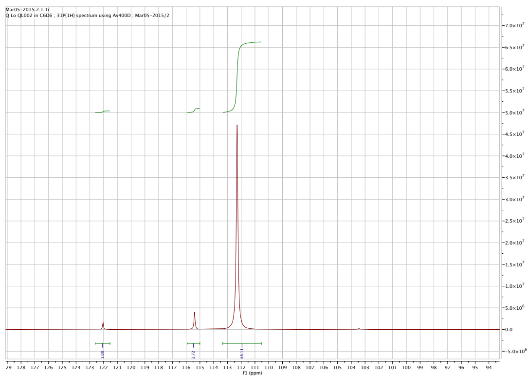
Figure S9. ^{31}P NMR spectrum of 1 in C_6D_6 at 298K (the signal at \delta = 115.4 ppm is bis(1,3-dimethyl-1,3,2-diazaphospholane)).
