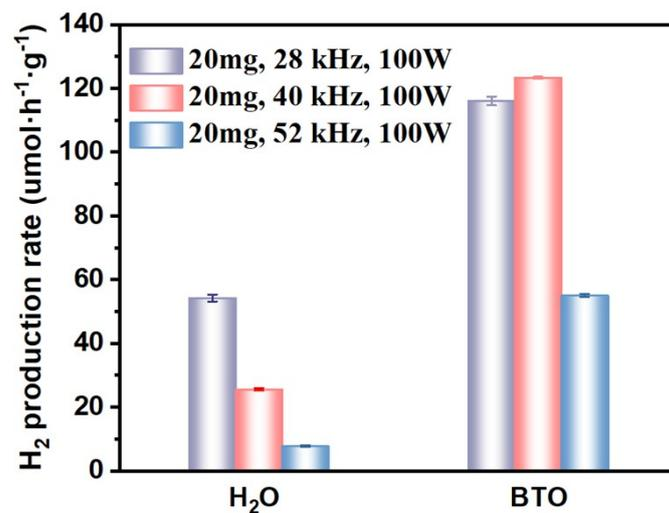
Fig. S3 The H<sub>2</sub> production rate under ultrasonic vibration of 100 W with different frequency over BTO.
