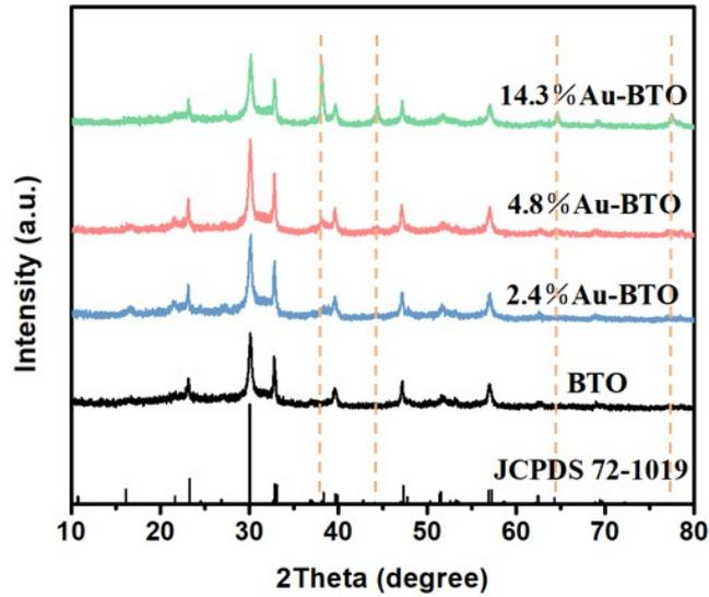
Fig. S1 XRD patterns of BTO, 2.4% Au-BTO, 4.8% Au-BTO and 14.3% Au-BTO.
