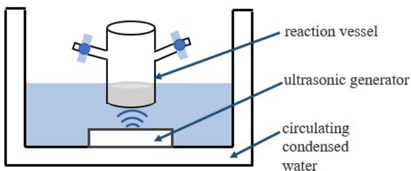
Fig. S9 Schematic diagram of piezocatalytic reaction unit.
