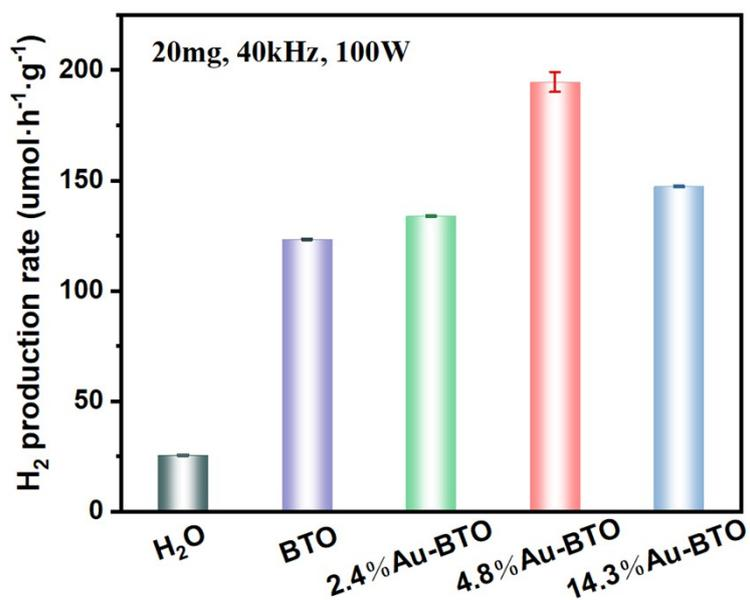
Fig. S4 The H<sub>2</sub> production rate of BTO, 2.4% Au-BTO, 4.8% Au-BTO and 14.3% Au-BTO under ultrasonic vibration of 40 kHz, 100 W.
