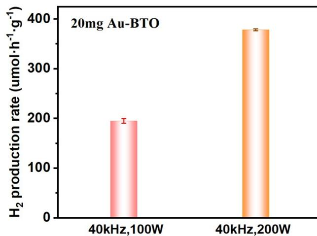
Fig. S7 The H<sub>2</sub> production rate under ultrasonic vibration of 40 kHz with different power over Au-BTO.
