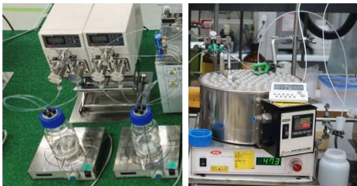
Figure S1. Photographs of flow reactor setup.
