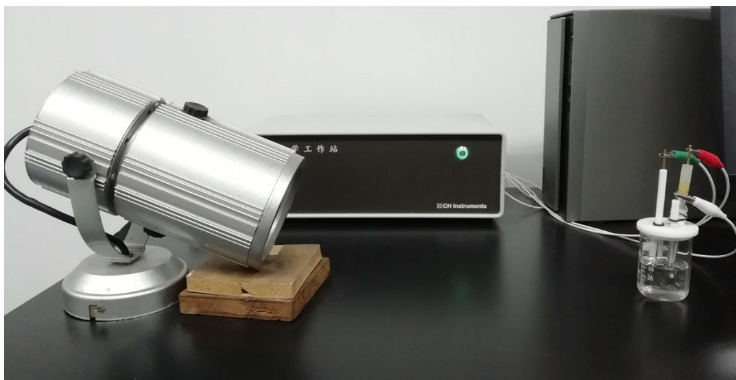
Fig. S8 the three-electrode system and the photoelectric properties measurement setup
