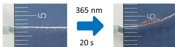
Fig. S26 The images showing the formation of the flexible joint under 365nm light irradiation.
