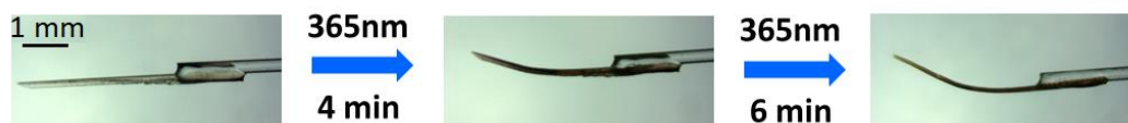
Fig. S21 Photomechanical bending photographs of Zn-Bpe-rod (4.50 mm × 0.30 mm × 0.20 mm) before and after irradiation by 365 nm light.
