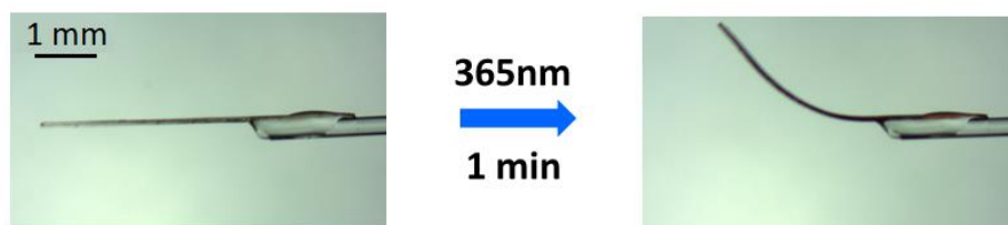
Fig. S20 Photomechanical bending photographs of Zn-Bpe-rod (3.50 mm × 0.20 mm × 0.10 mm) before and after irradiation by 365 nm light.
