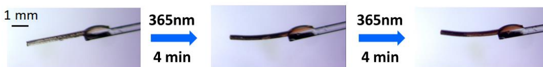
Fig. S22 Photomechanical bending photographs of Zn-Bpe-rod (4.10 mm × 0.35 mm × 0.34 mm) before and after irradiation by 365 nm light.
