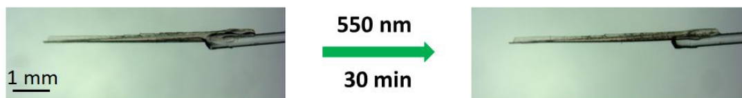
Fig. S16 Photographs of Zn-Bpe-rod (4.70 mm × 0.40 mm × 0.16 mm) before and after irradiation by 550 nm.
