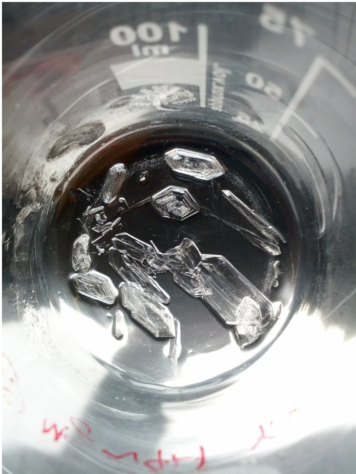
Figure S74: Photograph of \text{Sr}(\text{NH}_2\text{SO}_3)_2 \cdot 4\text{H}_2\text{O} as synthesised inside a 100 ml beaker (50 mm in diameter).
