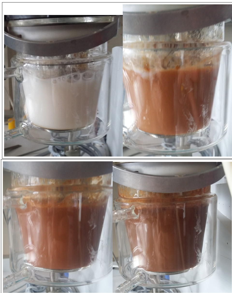
Figure S1: Color of the solution before (up left) and for various addition of \text{S}_2\text{O}_8^{2-} ( x = 0.12 (up right), 0.24 (down left) and 0.30 (down right)) in a R = 1.5 solution
