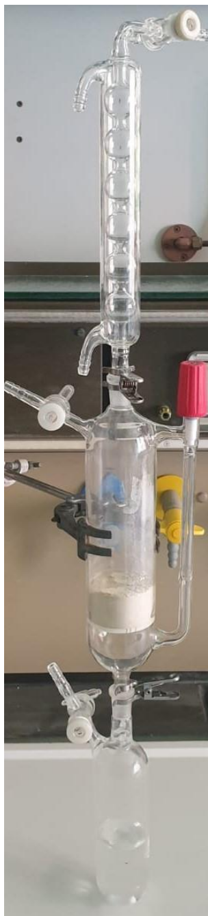
Photography S1: Schematic extraction apparatus with solvent flask (bottom), cooler (top), and vapor bypass (right).
