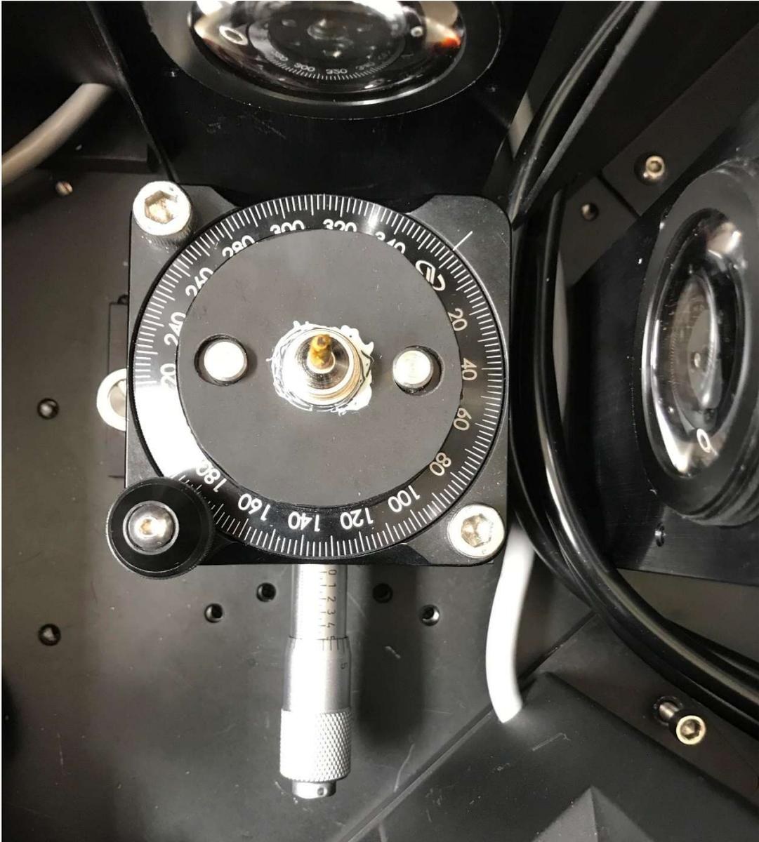
Figure S3. Position of loop platform in the spectrometer.
