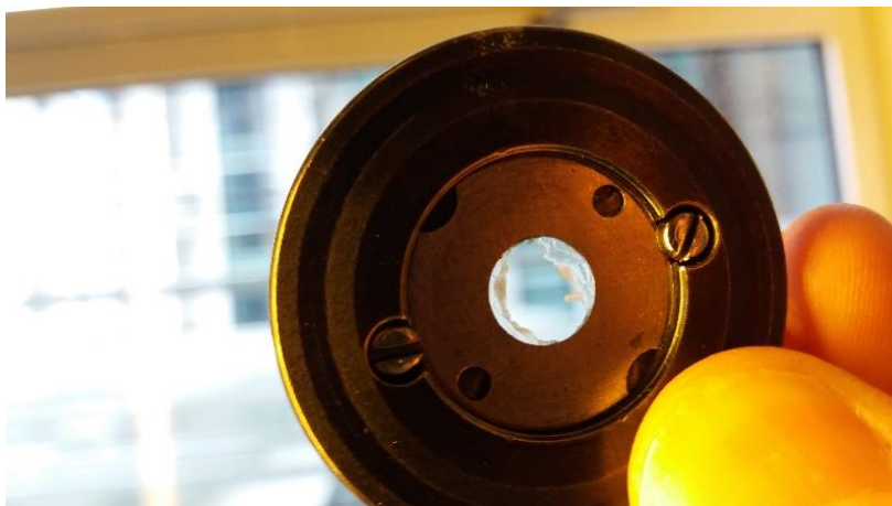
Figure S3. Destroyed polyacetate foil after 10 minutes contact of crystals of \text{H}_2[\text{B}_2(\text{SO}_4)_2] for PXRD.
