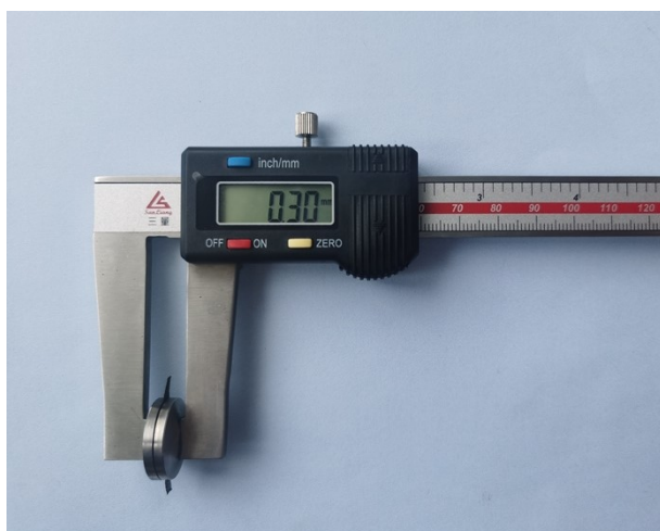
Fig. S9 The thickness measurement of the full-cell device by using vernier caliper.
