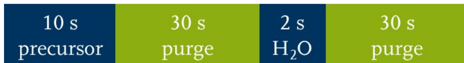
Figure S 7 Pulse and purge times of the ALD process schematically displayed.
