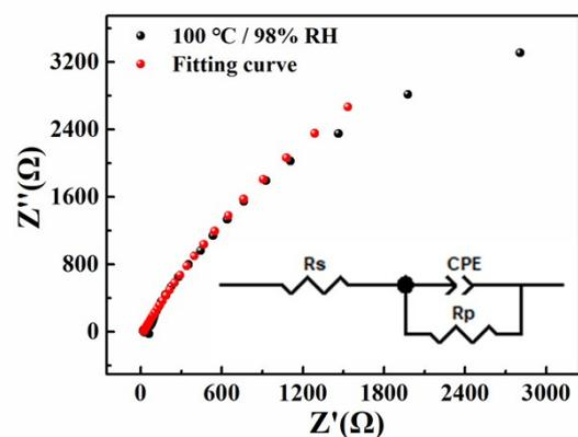
**Figure S10.** Nyquist plot of ZIF-90-SO<sub>3</sub>Na<sub>(2.3)</sub> measured at 100°C and 98% RH (black) and its fitting curve (red). The inserted diagram provides an equivalent circuit diagram for analyzing the Nyquist plot diagram.
