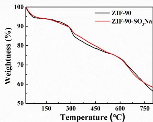
**Figure S3.** TGA curves of the ZIF-90 and ZIF-90-SO<sub>3</sub>Na<sub>(2,3)</sub>.
