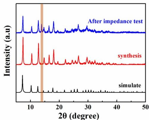
**Figure S8.** Powder X-ray diffraction pattern of ZIF-90 sample after AC impedance measurement at 98% RH.
