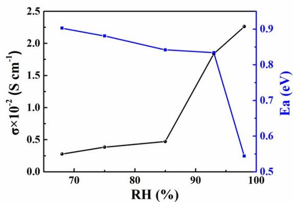
**Figure S12.** Proton conductivity at 100 °C and activation energy ( $E_a$ ) at different relative humidity (RH) of ZIF-90-SO<sub>3</sub>Na<sub>(2.3)</sub>.
