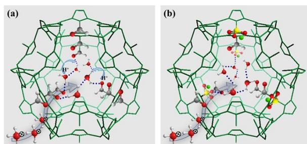
**Figure S11.** Diagram of the proton conduction path in ZIF-90 (a) and ZIF-90-SO<sub>3</sub>Na<sub>(2.3)</sub> (b) under high-humidity conditions.
