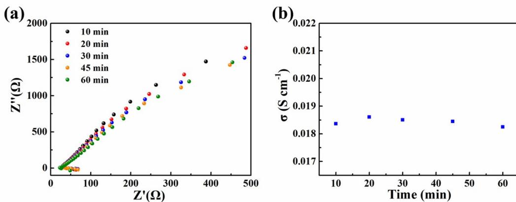
**Figure S5.** (a) Nyquist plot and (b) time-dependent conductivity plot of ZIF-90-SO<sub>3</sub>Na<sub>(2,3)</sub> at 100 °C and 93% RH.
