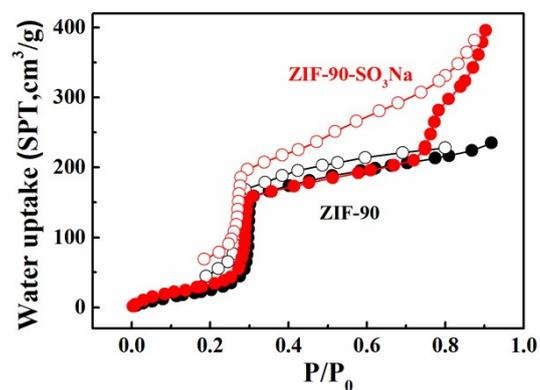
**Figure S6.** The water adsorption and desorption isotherm of ZIF-90 and ZIF-90-SO<sub>3</sub>Na<sub>(2.3)</sub>. (All tests were conducted at 25°C. Filled and open symbols represent adsorption and desorption, respectively.)
