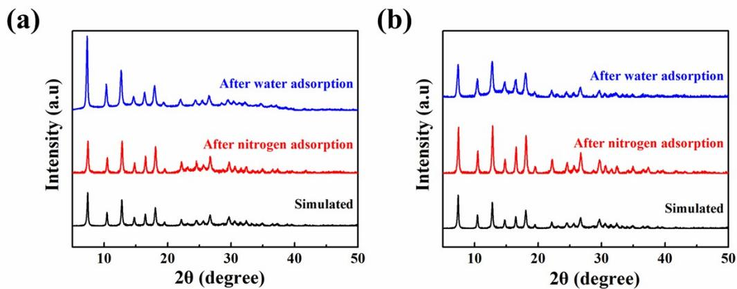
**Figure S4.** Powder X-ray diffraction patterns of (a) ZIF-90 and (b) ZIF-90-SO<sub>3</sub>Na<sub>(2,3)</sub> after N<sub>2</sub> and water vapor adsorption-desorption measurements.
