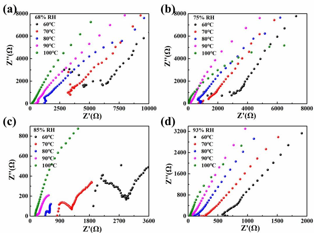
**Figure S9.** Temperature dependence of Nyquist plot for ZIF-90-SO<sub>3</sub>Na<sub>(2.3)</sub> at (a) 68% RH, (b) 75% RH, (c) 85% RH, and (d) 93% RH.
