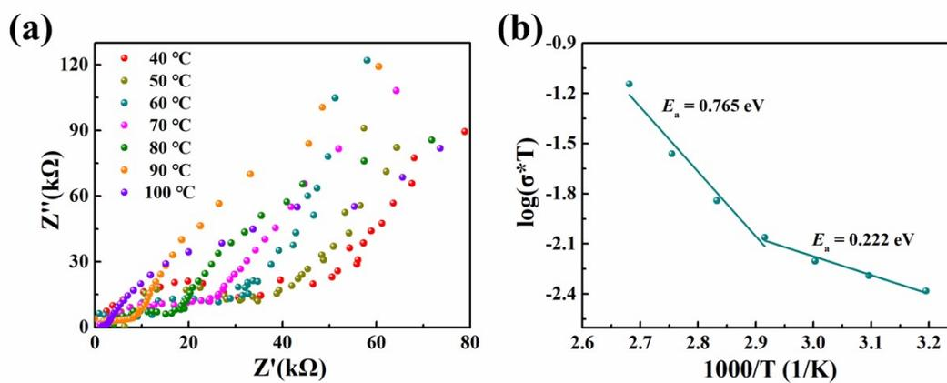
**Figure S7.** (a) Temperature dependence of Nyquist plot for ZIF-90 at 98% RH; (b) corresponding Arrhenius curve.
