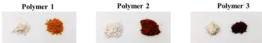
Figure S5: The precipitate of Hg-SCPs before and after iodine adsorption.
