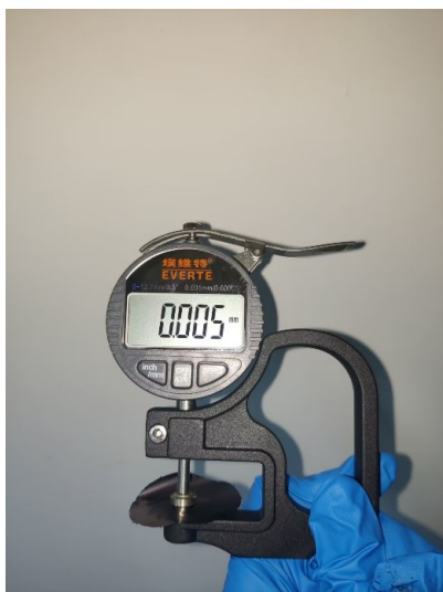
Fig. S8 The optical images showing the thicknesses of the pristine MXenes film (a) and the PK-MXenes film (b).
