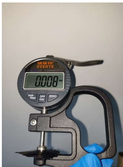
Fig. S8 The optical images showing the thicknesses of the pristine MXenes film (a) and the PK-MXenes film (b).
