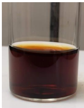
Fig S33. Dark red-brown solution generated upon bubbling of O 2 through a CH 3 CN solution of 13 for 8 h.
