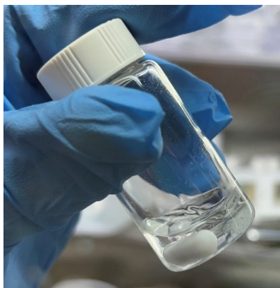
Figure S4. Digital image of 2 m (~1.3 M) LiFSI (first added) + 1 m (~0.6 M) LiTFSI in DOL-TTE after being placed for two weeks. This electrolyte shows a much higher viscosity than the Hybrid-DOL/PDOL-TTE. This comparison result illustrates the importance of the LiTFSI salt content.
