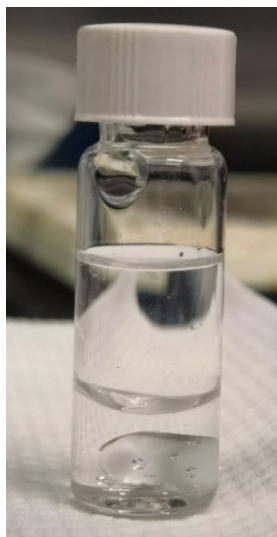
Figure S6. Digital image of the 2 m LiFSI triggered (fully polymerized for a long enough time) PDOL electrolyte (bottom) and TTE (top). The picture shows that the fully polymerized PDOL cannot be dissolved in the TTE, forming a solid-liquid separation state.
