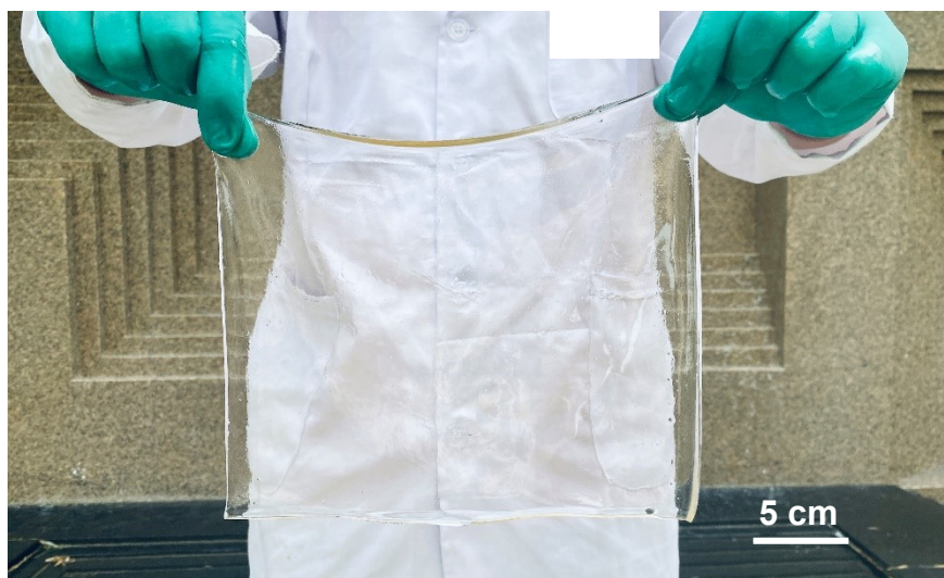
Figure S7. Large-scale production of the CP/EGZn/betaine hydrogel electrolyte.
