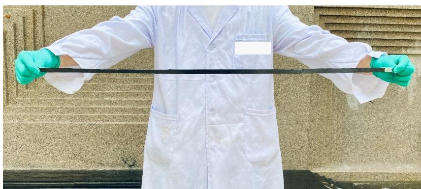
Figure S24. Metre-scale ZIC tapes made of the CP/EGZn/betaine hydrogel electrolytes that sandwiched between Zn sheet and cc.
