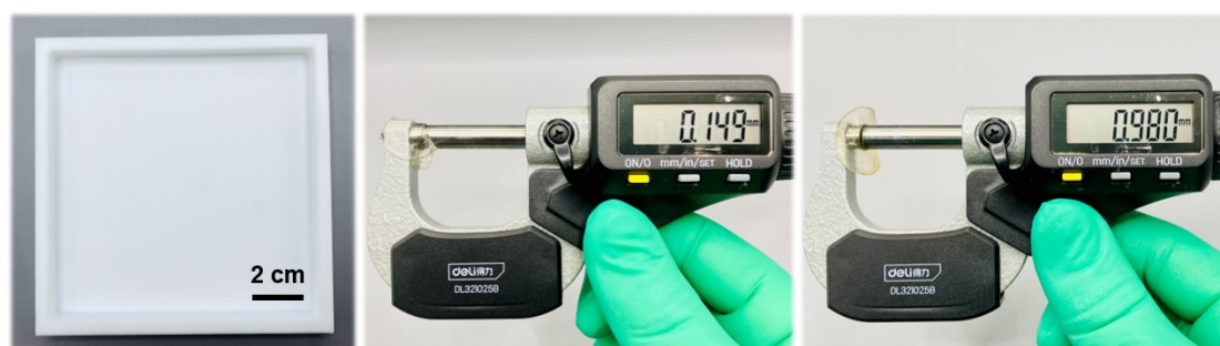
Figure S63. A customize mold is used to tailor the thickness of a hydrogel specimen.
