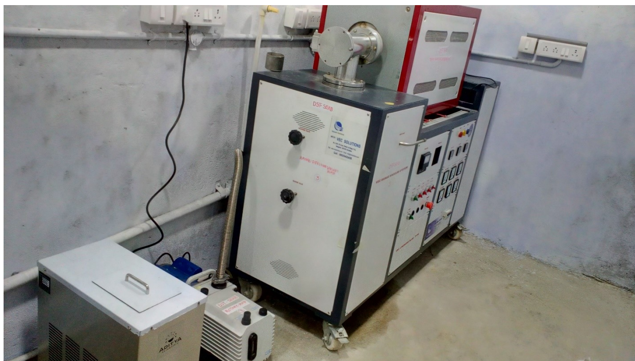
Figure S24 High vacuum furnace for incineration of solid-waste obtained from industrial raw wastewater.
