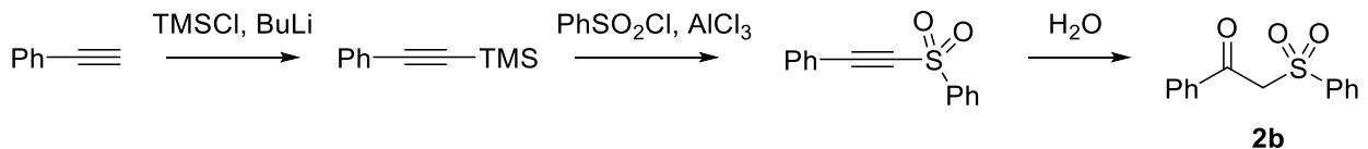
$$\text{Atom economy} = \frac{M(2b)}{M(\text{PhC}\equiv\text{CH}) + M(\text{TMSCl}) + M(\text{BuLi}) + M(\text{PhSO}_2\text{Cl}) + M(\text{AlCl}_3) + M(\text{H}_2\text{O})} \times 100\% = 43\%$$
