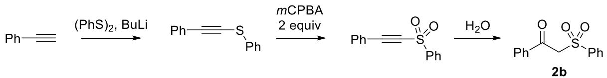
$$\text{Atom economy} = \frac{M(2b)}{M(\text{PhC}\equiv\text{CH}) + M(\text{PhSSPh}) + M(\text{BuLi}) + 2M(m\text{CPBA}) + M(\text{H}_2\text{O})} \times 100\% = 35\%$$
