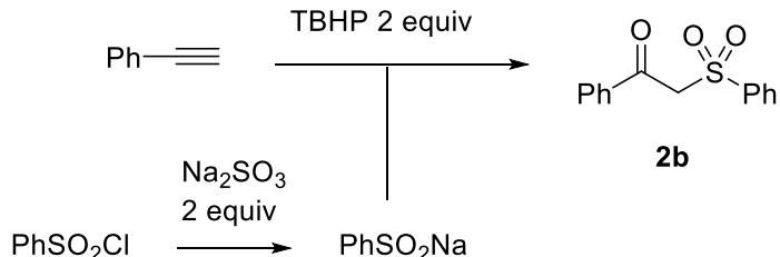
$$\text{Atom economy} = \frac{M(2b)}{M(\text{PhC}\equiv\text{CH}) + M(\text{PhSO}_2\text{Cl}) + 2M(\text{Na}_2\text{SO}_3) + 2M(\text{TBHP})} \times 100\% = 37\%$$
