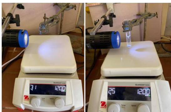
Figure S1. A. Experimental setup of the photocatalyst-free aerobic oxidation of aldehydes to carboxylic acids using Kessil PR160L-370 nm. B. Experimental setup of the photocatalyst-free aerobic oxidation of aldehydes to carboxylic acids under sunlight.
