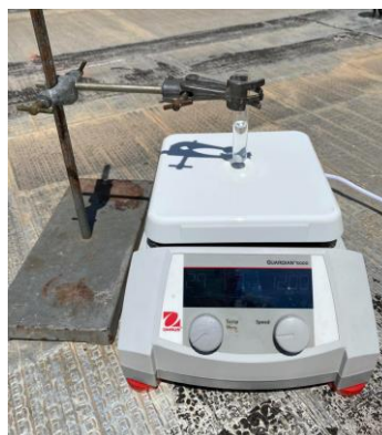
Figure S1. A. Experimental setup of the photocatalyst-free aerobic oxidation of aldehydes to carboxylic acids using Kessil PR160L-370 nm. B. Experimental setup of the photocatalyst-free aerobic oxidation of aldehydes to carboxylic acids under sunlight.
