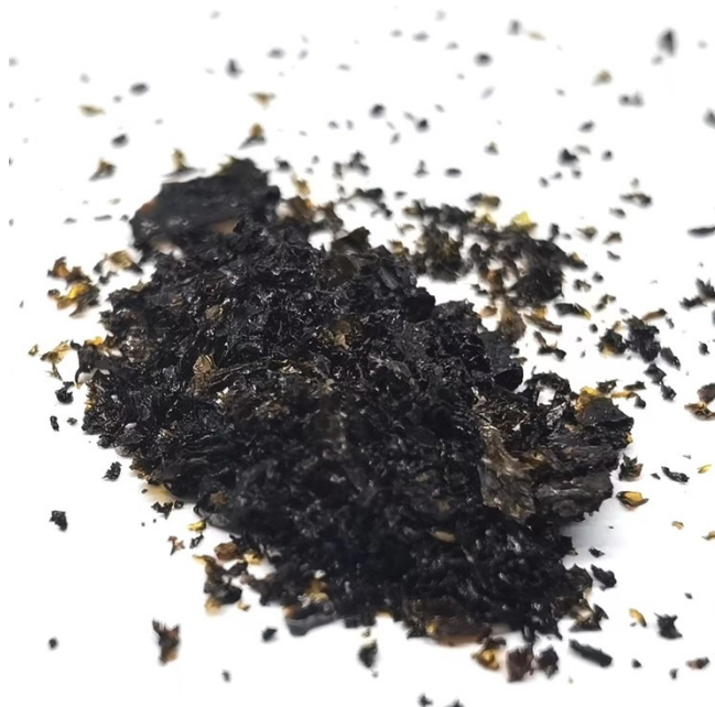
Fig. S2 Appearance of aminated lignin (120EL), which presents in a brown to black sheet-like solid form.
