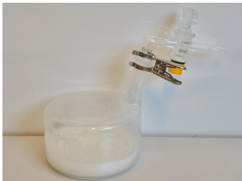
Figure S39: Flat-bottomed glass vessel charged with 100 g \text{Ph}_3\text{P} .
