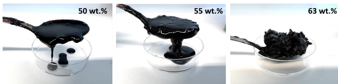
Figure S2: Visual appearance of LS-SKL (5 to 1 w/w) mixtures in 2 M NaOH at different total lignin concentrations.
