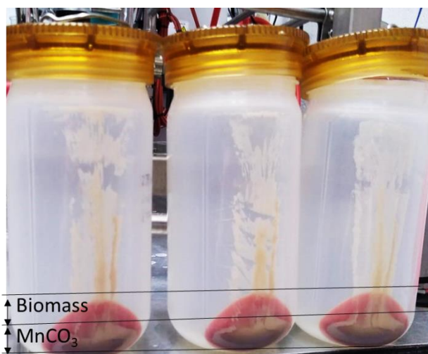
Fig. S11 Bioprecipitated Mn as \text{MnCO}_3 (beige layer) below the biomass layer (pink) after centrifugation to separate the solid and dissolved fractions.
