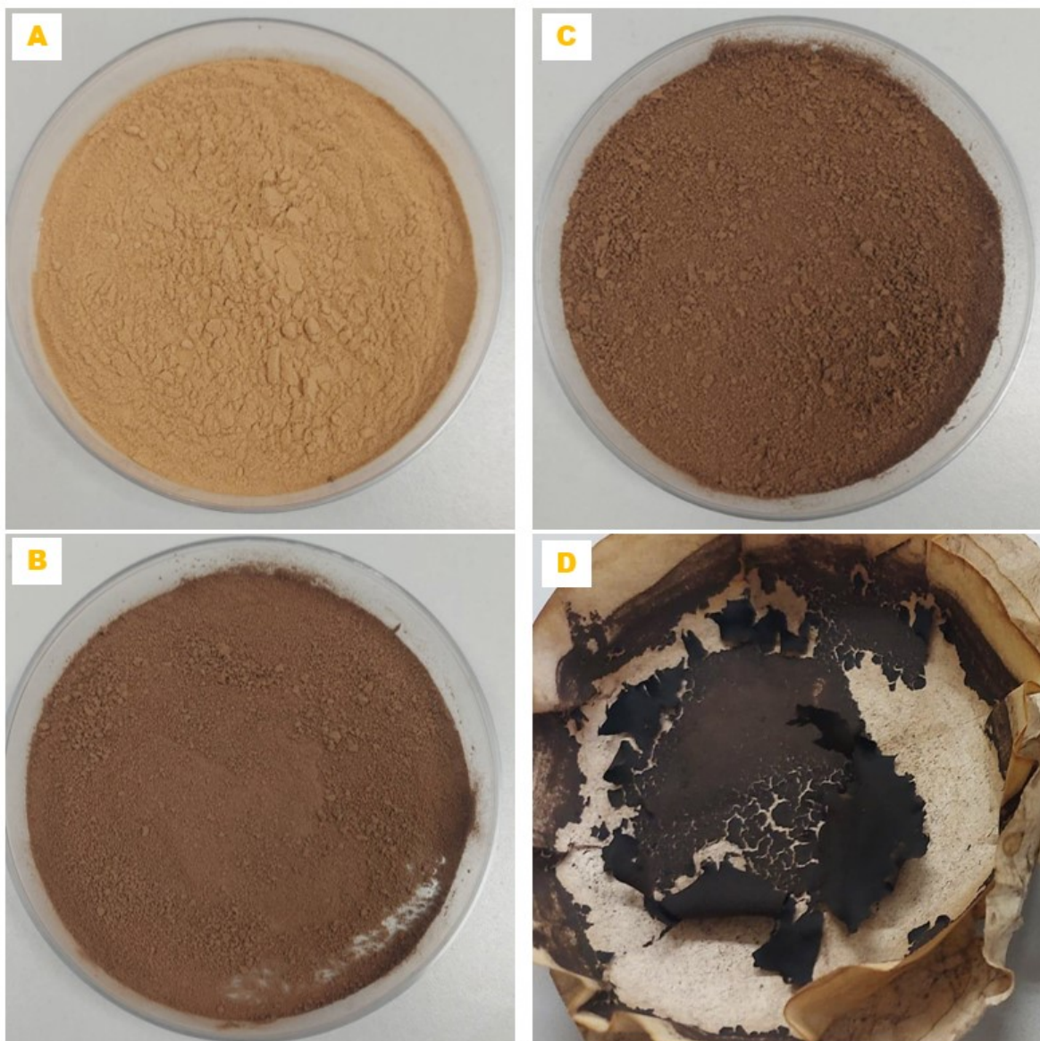
Fig. SF1 Photos of the original cork biomass (A) in comparison with the UFC-2 (B) and UFC-3 (C) solid hydrolysis products and the carbohydrate-lignin complex after suberin extraction (D)
