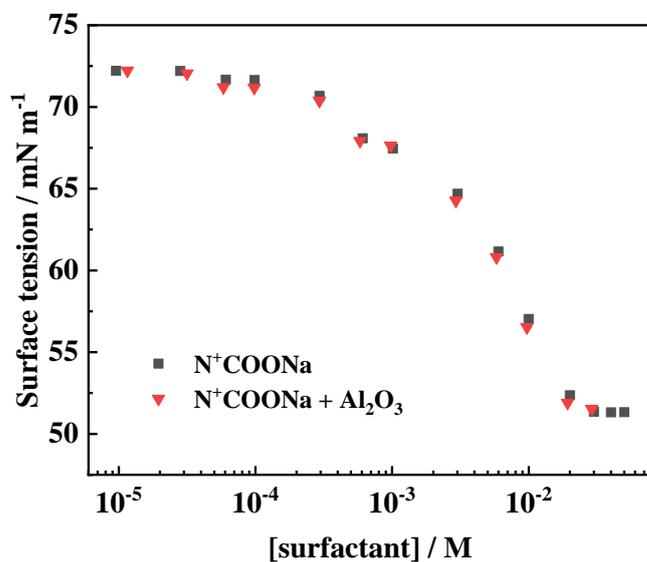
**Figure S9.** The surface tension of N<sup>+</sup>COONa solution before and after addition of alumina particles.
