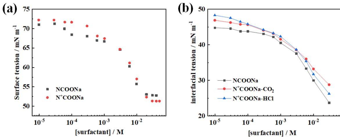
**Figure S1.** Surface tension (a) /interfacial tension (b) curves of NCOONa/N<sup>+</sup>COONa at different concentrations
