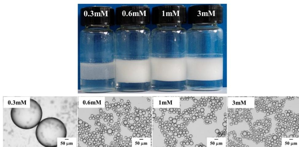
**Figure S6.** The photos of the Pickering emulsions (*n*-octane/water) prepared from NCOONa and 0.1 wt.% alumina particles after five months of stabilization: from left to right NCOONa concentrations are: 0.3, 0.6, 1, 3 mM.
