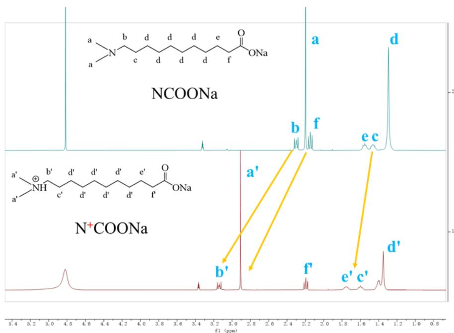
**Figure S3.** <sup>1</sup>H-NMR spectrum of NCOONa before (upper) and after (lower) bubbling CO<sub>2</sub> (CD<sub>3</sub>OD/D<sub>2</sub>O).
