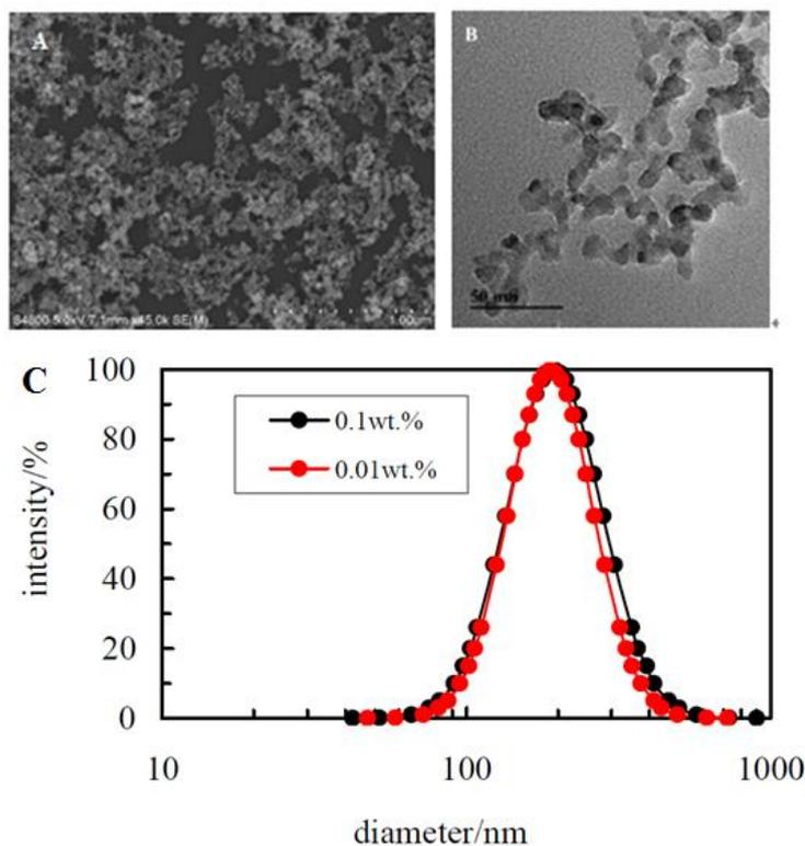
**Figure S5.** (A) SEM and (B) TEM images of alumina nanoparticles and (C) size distribution of 0.1 wt.% and 0.01 wt.% alumina nanoparticles dispersed in pure water by ultrasonication at neutral pH (~6.8) at 25 °C. The z-average diameter of the particles in water after ultrasonication is ~ 192 nm.
