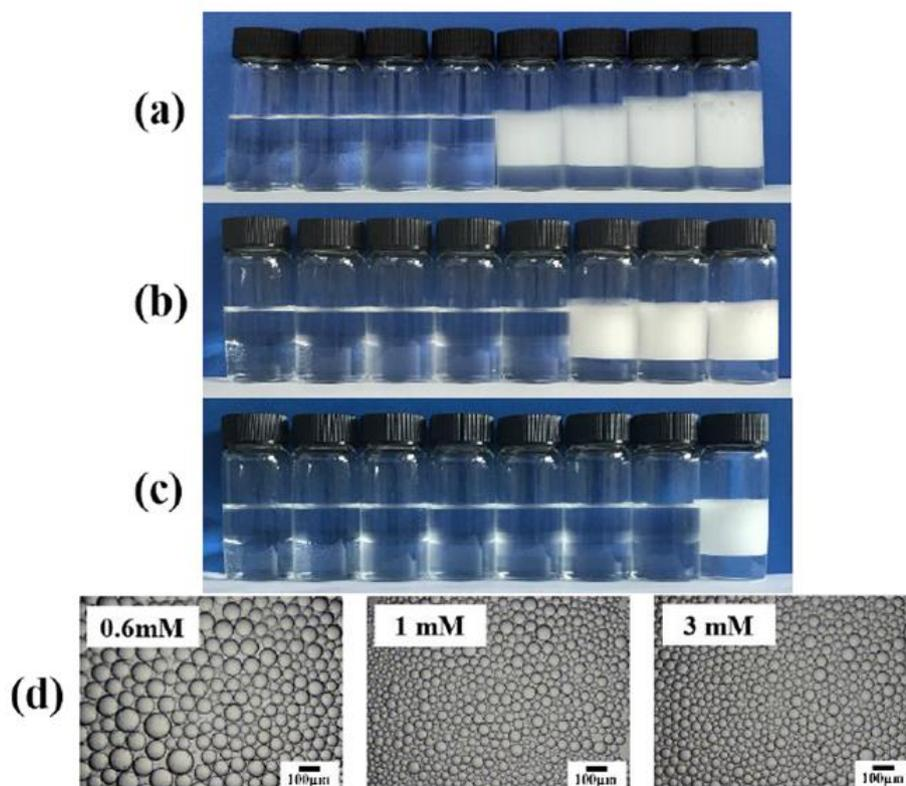
**Figure S4.** Photos of emulsions (*n*-octane/water) prepared by NCOONa at different concentration (from left to right for a and b): 0.01, 0.03, 0.06, 0.1, 0.3, 0.6, 1, 3 mM and as shown for (d), taken (a) immediately, and (b and d) 24 h, and (c) 48 h after preparation.
