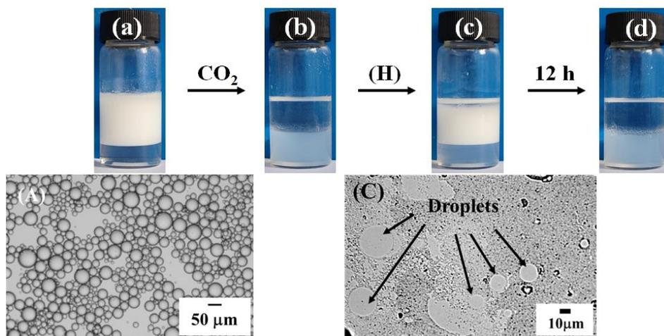
**Figure S10.** The photos and selected micrographs of the emulsion. (a) the emulsion stabilized by NCOONa (0.6 mM) and alumina particles (0.1 wt.%); (b) demulsification after bubbling CO<sub>2</sub>; (c) the emulsion stabilized by N<sup>+</sup>COONa and alumina particles after re-homogenization (b); (d) photo of (c) taken 12h after preparation. (A) micrographs of the emulsion in (a); (c) micrographs of the dried emulsion in (c).
