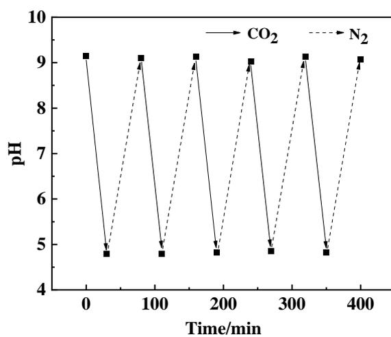
**Figure S2.** The pH value of NCOONa solution (0.3 mM) after bubbling CO<sub>2</sub> and N<sub>2</sub> alternately.
