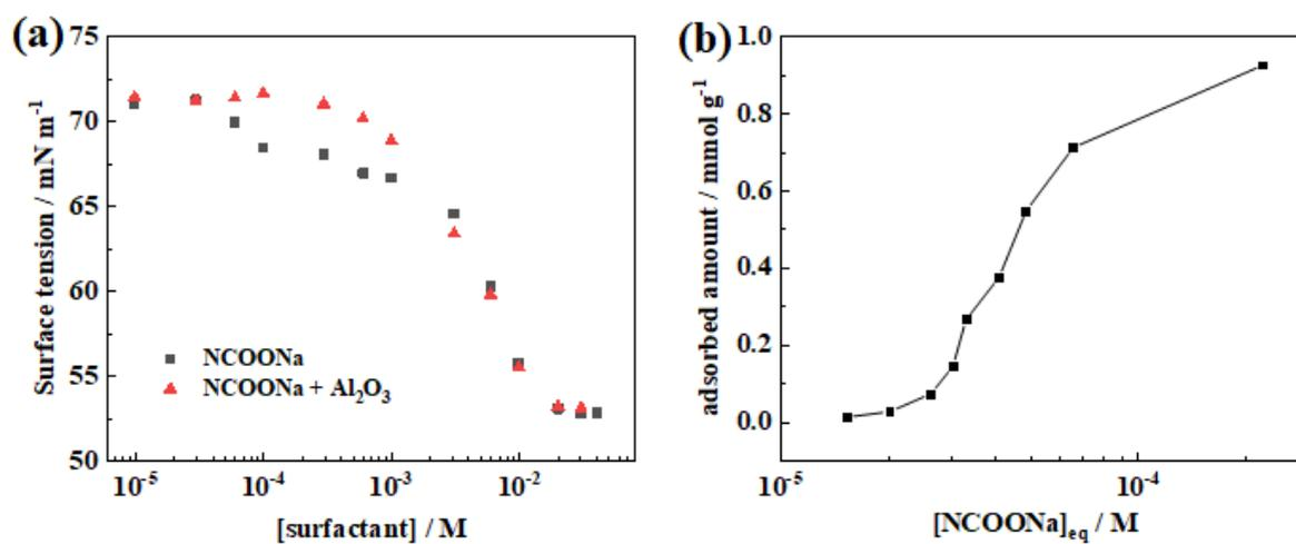
**Figure S8.** (a) The surface tension curves of NCOONa solution before and after adding alumina particles, (b) The curve of the adsorbed amount of NCOONa on the surface of alumina particles as a function of the equilibrium concentration of NCOONa in solution.
