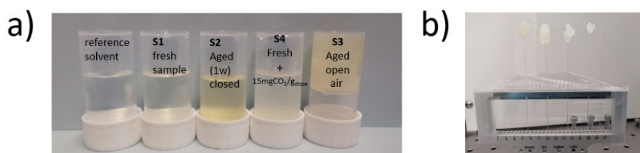
Figure S10 -Samples appearance before SAXS/WAXS experiments. a) samples in bottle containers. b) samples located at the SAXS/WAXS sample holder
